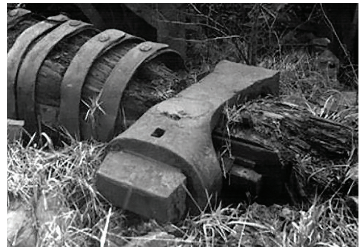
A tilt hammer with its rotten oak shaft
